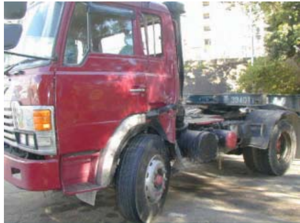
Figure 3.4 – The damaged driving cab of the container truck
