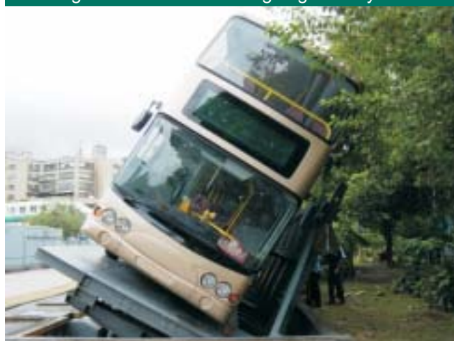
Figure 8.6 – A bus undergoing stability test
