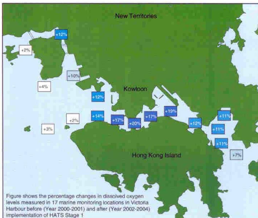
Figure 1: Changes in dissolved oxygen levels after implementation of HATS Stage 1
