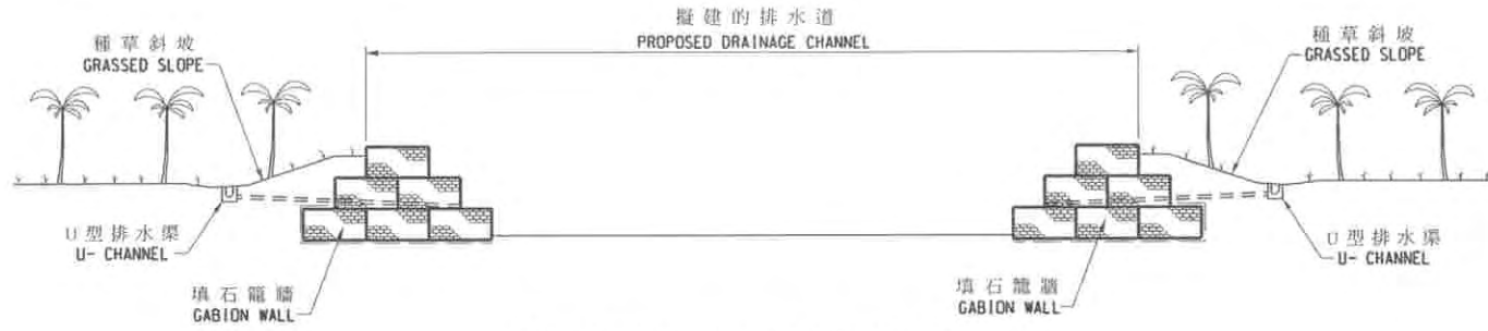
排水道典型橫切面 TYPICAL SECTION OF GABION WALL CHANNEL 不依比例 NOT TO SCALE
