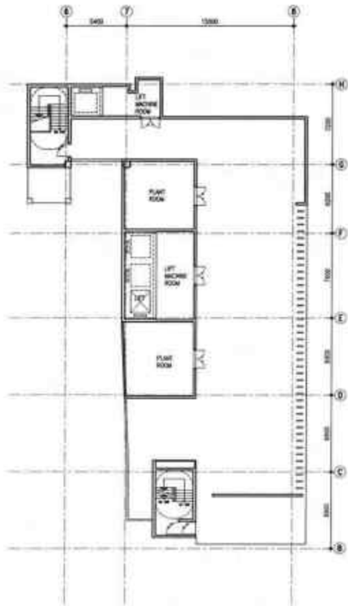
SERVICES FLOOR PLAN (8TH FLOOR)
