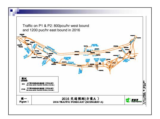
One traffic lane can usually accommodate 1000 pcu/hr, the amount of predicted traffic demand can easily be met by one lane west bound and two lanes east bound; So the 2x2 lane P2 design is more than adequate.
