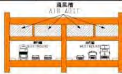
典型明挖回填式隧道橫切面 TYPICAL SECTION FOR CUT-AND-COVER TUNNEL 不按比例 N.T.S.
