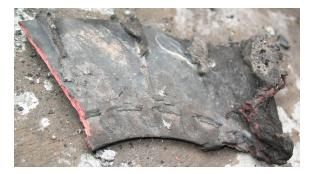
Once the wirings and rubber hoses hit by the sparks were ignited, fire flames spread to other parts of the engine compartment, and up through the air-conditioning ducts, and so the rear bus body was severely burnt.
