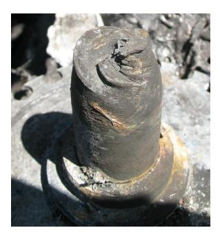
A steel shaft will only twist off in a ductile manner under extremely high temperature when the material is softened.
