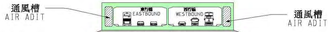
典型海底隧道橫切面 TYPICAL SECTION FOR UNDERWATER TUNNEL 不按比例 N.T.S.
