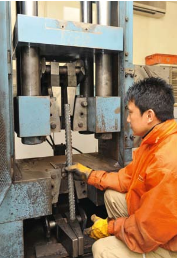
Tensile strength test on carbon steel reinforcing bar
