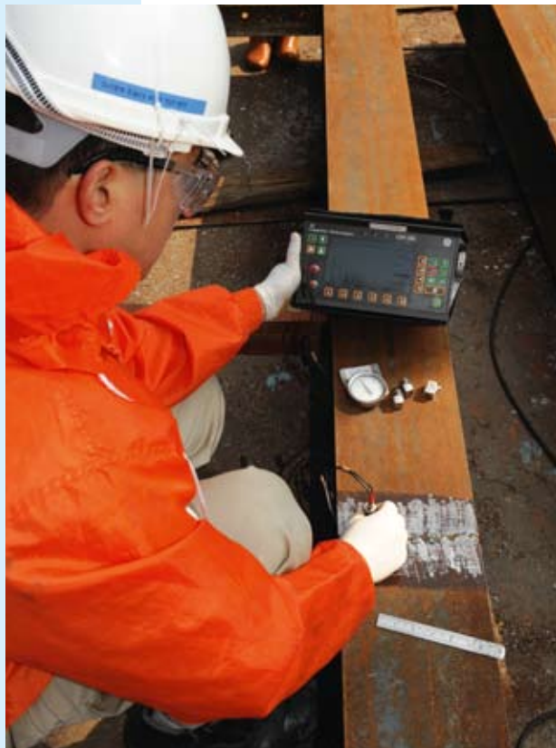
Internal defect inspection of 'I' beam connection joint
