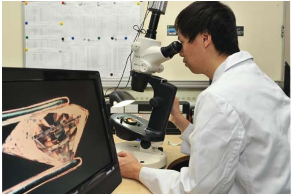
Inspecting laser inscription on a diamond
