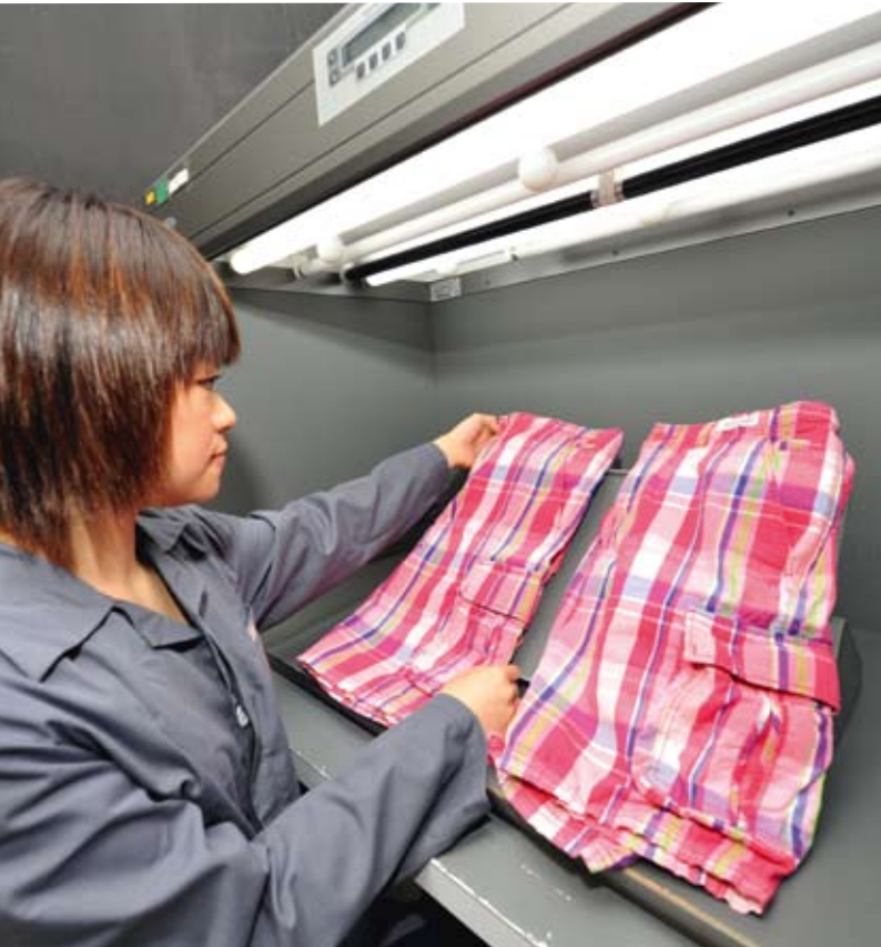
Appearance assessment of textile products after washing and drying
