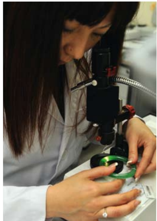
Analysis of Fei Cui (Jadeite Jade) bangle using Visible Light Spectroscope
