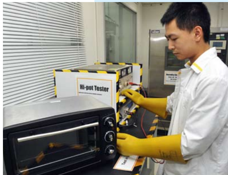
Electric strength test for an electric oven to ensure consumer safety
