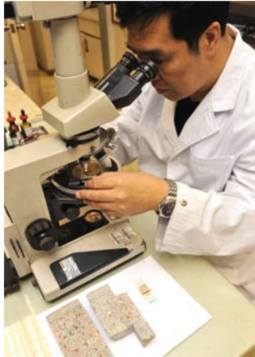
Petrographic examination to evaluate concrete quality
