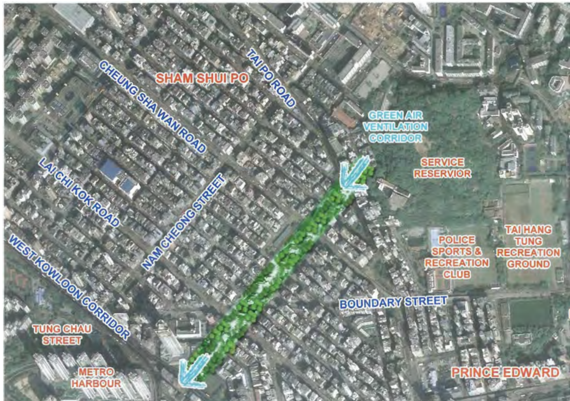
Figure 8.2: This conceptual image illustrates the possibility of creating a linear park through Sham Shui Po by removing existing buildings and linking existing open sites. This would help reduce the deficit of public open space, green a densely developed area of the city, provide an air ventilation corridor, reduce population density and help reduce the Urban Heat Island Effect.
