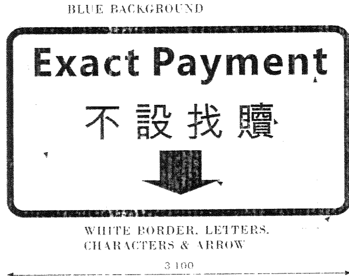
No Change Toll Sign
