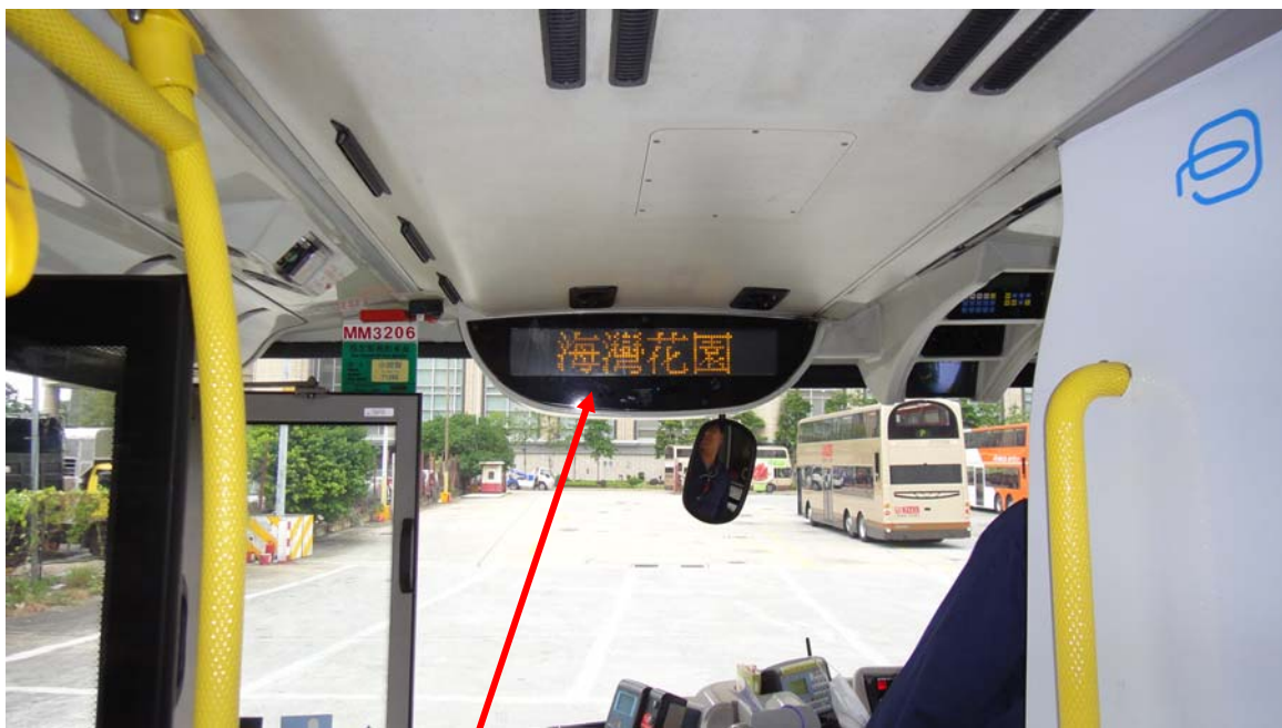
Photograph 9 : On-board bus stop announcement display panel 相片九：車廂內的報站顯示屏
