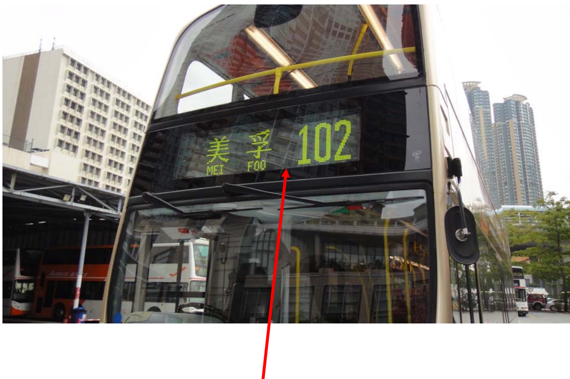
Destination and route number display panel on the front 車前方的終點站及路線編號顯示屏
