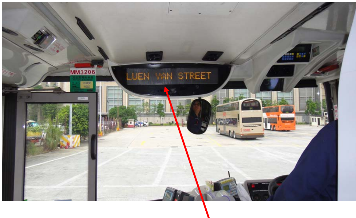
Photograph 10 : On-board bus stop announcement display panel 相片十：車廂內的報站顯示屏
