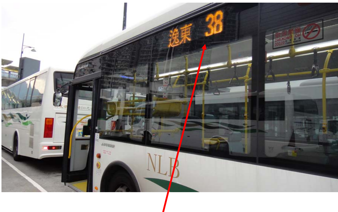
Route number display panel on the side 車身側面路線編號顯示屏
