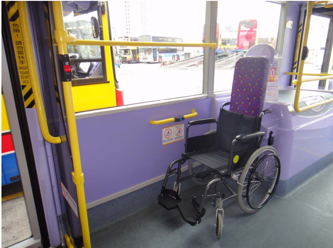
Photograph 2 : Wheelchair space with backrest and restraint lap belt 相片二：附設靠背及安全索帶的輪椅停放處
