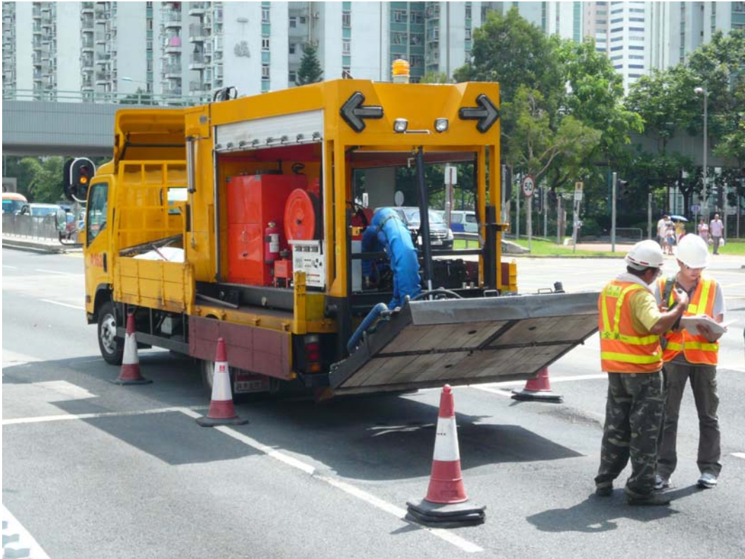
[Figure 3] Road maintenance workers are arranging localized repair by small-size thermal patcher
