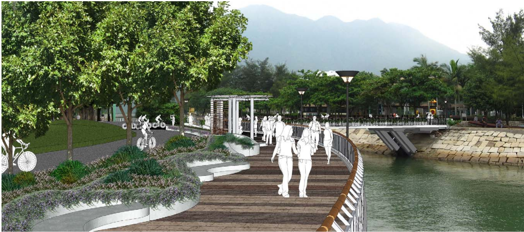
支撐面板行人道連單車徑(構思圖) PEDESTRIAN WALKWAY ON SUSPENDED DECK AND CYCLE TRACK (ARTIST'S IMPRESSION)
