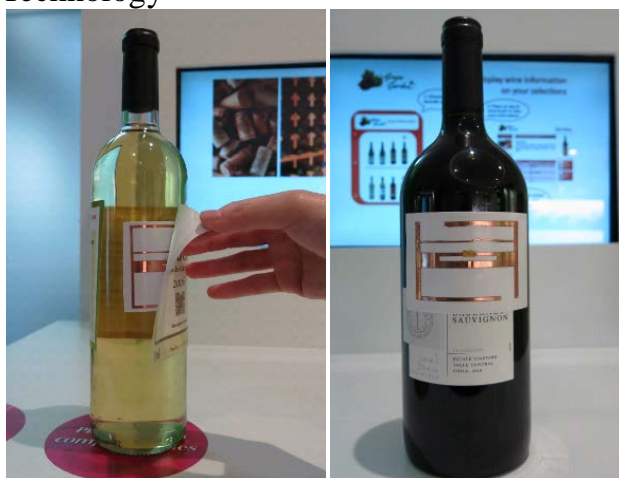
LSCM's antenna design for wine bottles
