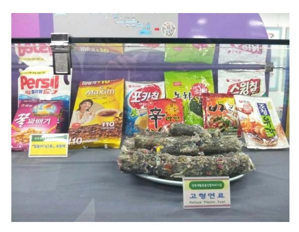
Plastic waste converted into "refuse plastic fuel" for energy production
