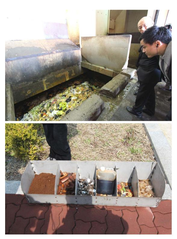
Recycling of food waste into different resources using anaerobic digestion technology. The resultant materials are: (from left) animal feed, bones, steel utensils, biodiesel, recycled residuals, and wooden chips
