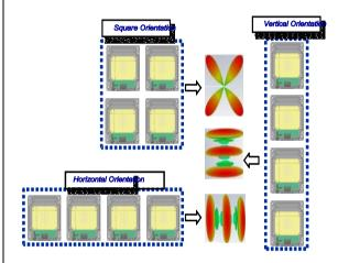
Example Active Antenna System Configuration (top) and Example Beam Forming (bottom)
