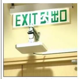
RFID reader installed at care centre's checkpoints
