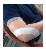
This project solves the technical problem of adhesive tapes currently in the market. HKRITA has developed a re-peelable elastic tape containing an elastic polymer micro-fabricated with the biomimetic nano- or micro- surface pattern. The pattern is inspired by climbing insects' attachment mechanism. The tape has achieved good adhesion and removal from the skin.
