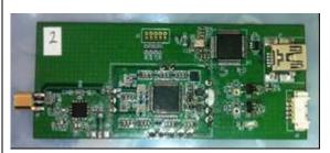
RFID reader device using LSCM Lightweight RFID Reader Chip
