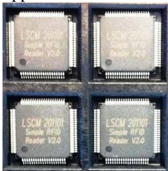
LSCM's UHF Gen2 Reader Chip for mobile RFID applications - first reader-chip ever designed in Greater China region
