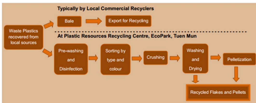
FIGURE 3.4 Flow Diagram of Plastic Recycling Processes in Hong Kong 13
