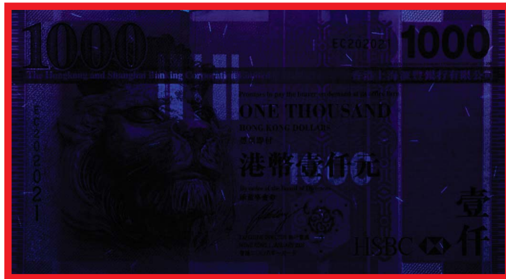
Counterfeit note: dull and unclear fluorescent barcode
