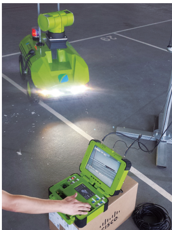
The Surveillance Patrol Robot of Smart Cities (Hong Kong) Limited operated at Car Park Building for functionality testing
