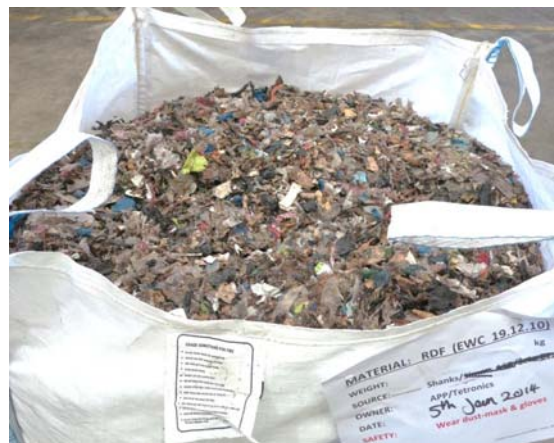
Members were briefed on the making of Refuse Derived Fuels which consisted of the combustible materials in MSW
