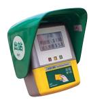
設在輕鐵月台上的出站收費器 已加裝發聲器,報讀從八達通 扣除的車費及其餘額,切合視 障乘客的需要。此外,所有輕 鐵月台的出站/入站收費器,查 閱機及增值機亦已配備資訊點 字板。 Exit Fare Processors at Light Rail Stops have Audible Devices, which provide audible Octopus readings for visually impaired passengers. Information in Braille is also provided at all Light Rail Exit/Entry Fare Processors, Enquiry Processors and Add Value Machines.
