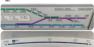
Flashing System Maps showing the current and next station, direction of the train and the side the doors will open for exiting passengers are provided in all trains on the Kwun Tong Line, Tsuen Wan Line, Island Line and Tseung Kwan O Line.
