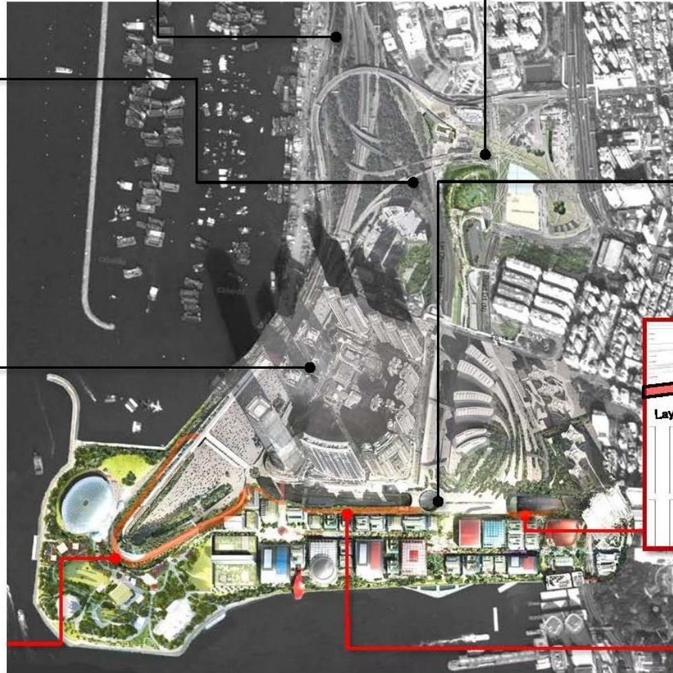
Scheme 2 計劃 2 Proposed single lane elevated road connecting elevated Nga Cheung Road to toll plaza of WHC 擬建高架單線行車道連接雅翔道高架路段至西區海底隧道收費廣場
