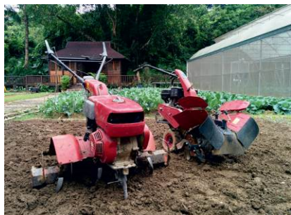
1. Cultivator tiller To loosen top soil before cultivation.
