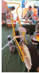
13. Planter For precise seeding directly onto the soil bed.
