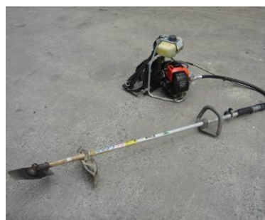
6. Brush cutter To clear grass, small bushes and undergrowth.
