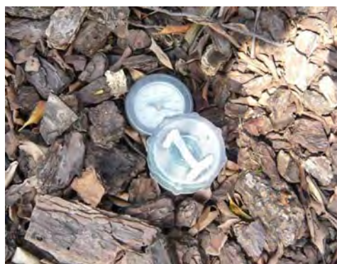
Photo 6 - Tensiometer installed in root zone to monitor soil moisture
