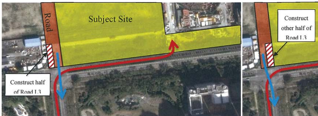
Figure 6.1: Road L3 construction to enable constant access
