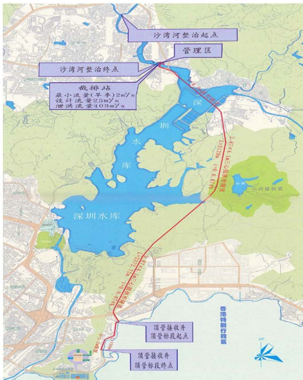
Figure 5 — General layout plan of the Basin Sewage Interception Works System at Shenzhen Reservoir
