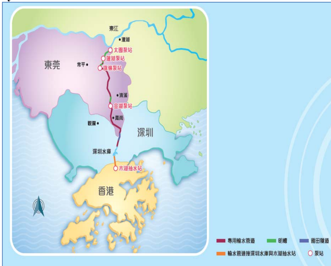
Figure 2— Water Conveyance Route of the Dongshen Water Supply System
