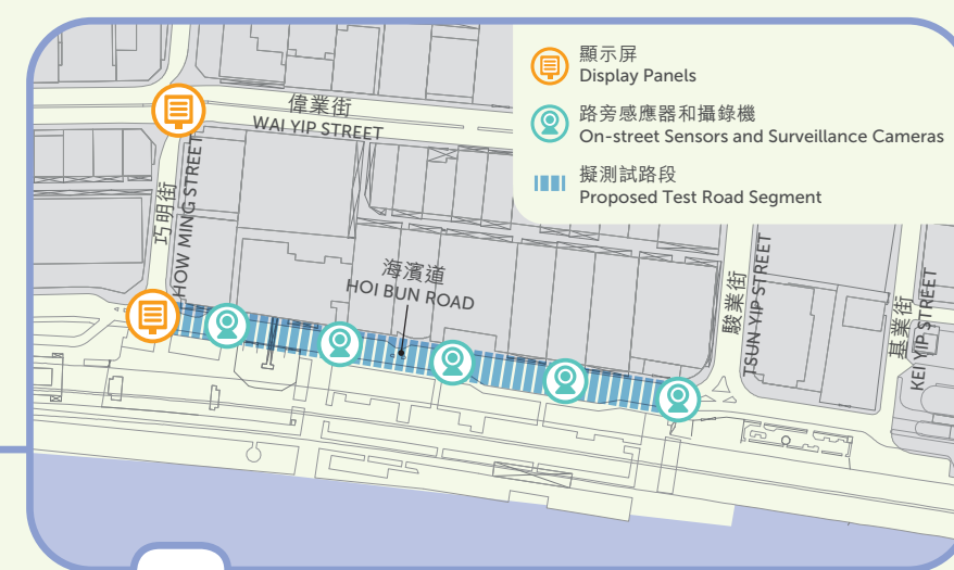
路旁落貨區監測系統 Kerbside Loading/Unloading Bay Management System
