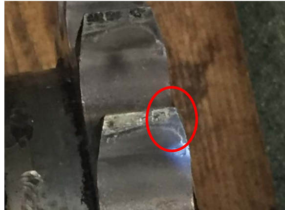
Figure 8: Photo of wear surface on the teeth of motor sprocket
