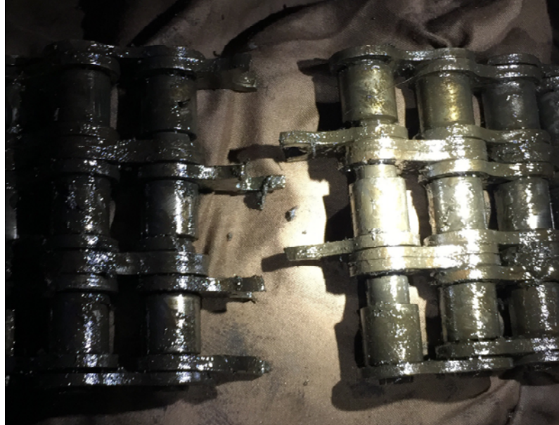
Figure 4: Photo showing the breakage position of main drive chain
