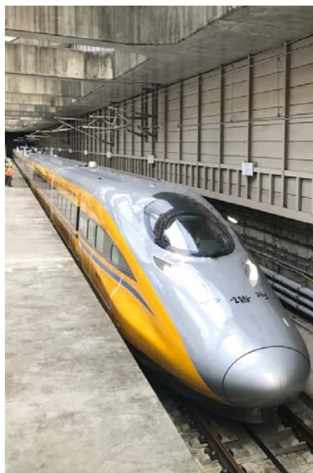
The Comprehensive Inspection Train inspects the railway infrastructure and systems
