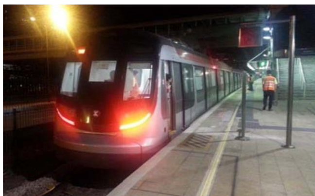
Dynamic test of new trains on the EAL during non-service hours
