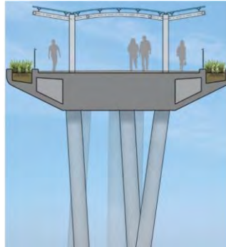
LW-02高架行人道 典型橫切面 Elevated Walkway LW-02 Typical Section
