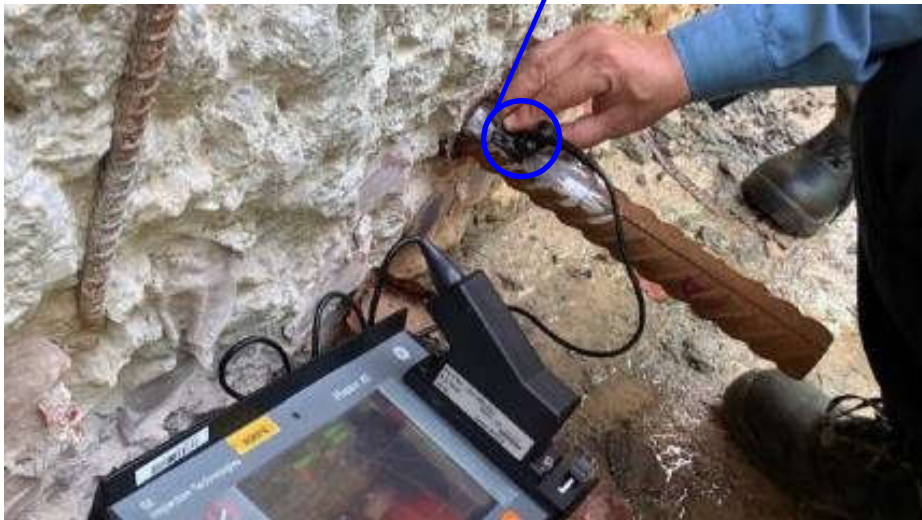
將探測器放上鋼筋接觸面 Put the detector on the steel bar surface
