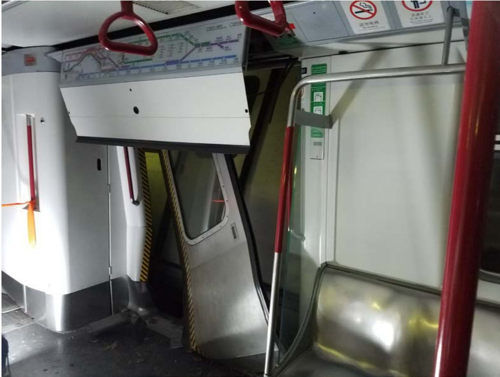
Figure 2: Damage to the saloon of train T112
