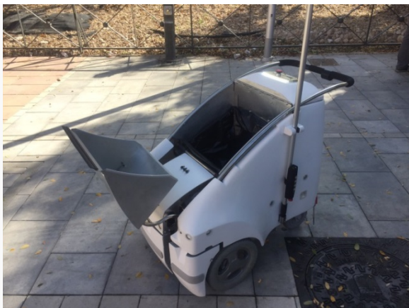
Figure 4 – A1A3 automated trolley
