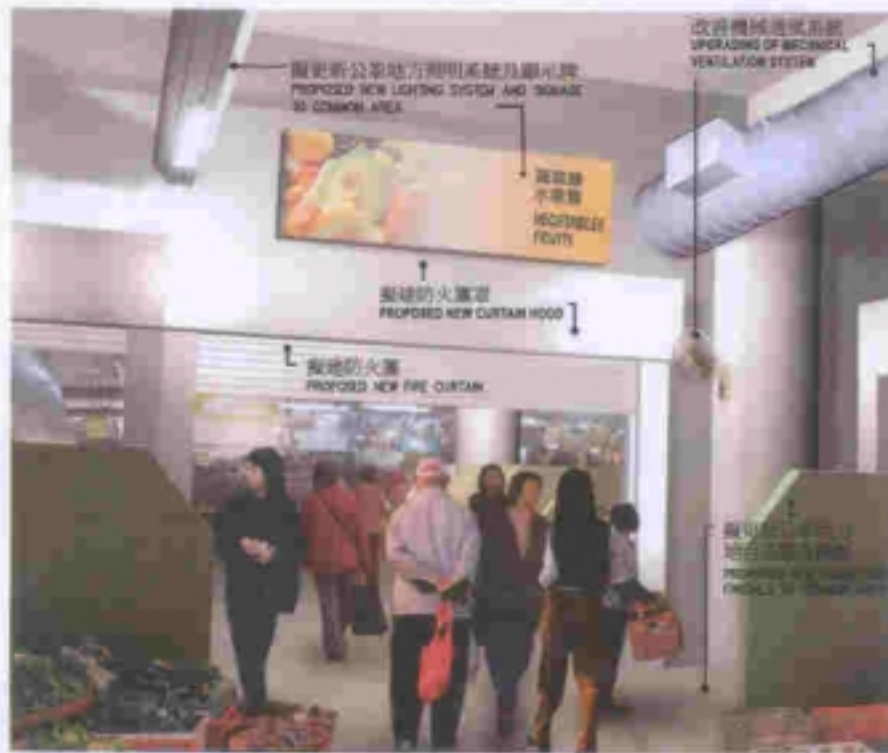
擬改善工程電腦效果圖 COMPUTER RENDERED DRAWING FOR PROPOSED IMPROVEMENT AND UPGRADING WORKS
