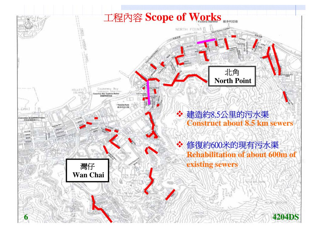
灣仔東部及北角污水收集系统 – 餘下工程 Wan Chai East and North Point Sewerage, Remaining Works
