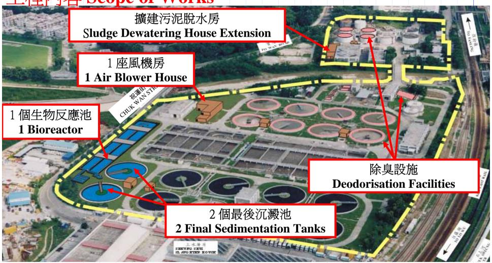
❖擴建現有的污水處理廠以提升污水處理量由每日80 000立方米至93 000立方米 Expand the existing treatment works to increase the treatment capacity from 15 80,000m<sup>3</sup>/day to 93,000m<sup>3</sup>/day
