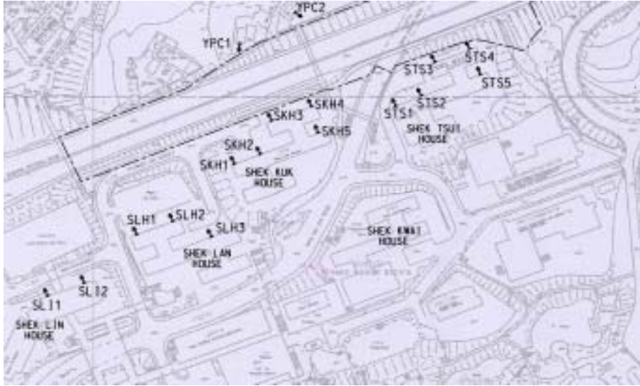
(灰色陰影的數字顯示在某該噪音感應強的地方，全部吸音板的減音交效果較全部反音板為佳) (NSRs where absorptive panels are more effective than reflective panels are shaded in grey)
