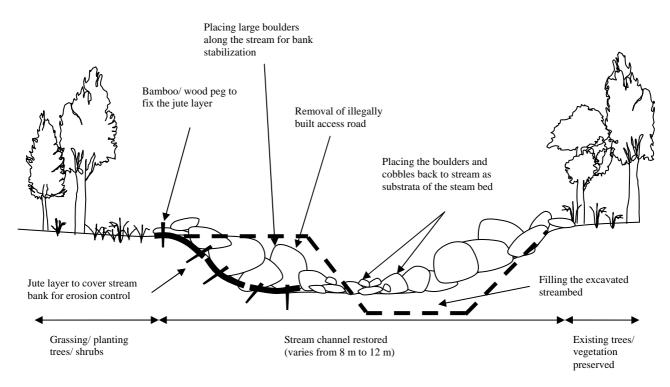
Note : The dotted line represents the cross section of the stream after disturbance
