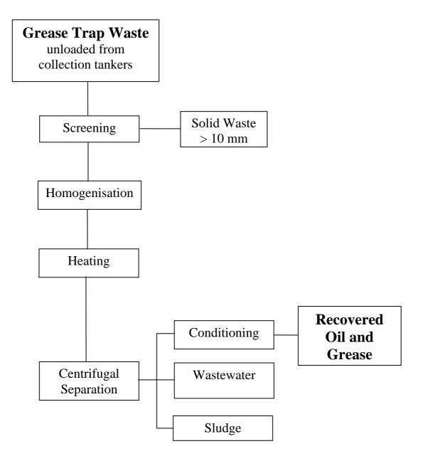
(Note : For the current intake of GTW of 400 tonnes per day, about 15 tonnes per day of concentrated oil and grease will be recovered. The balance is mostly water.)
