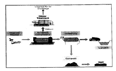
Fig.6 Process flow diagram of In-vessel Composting
