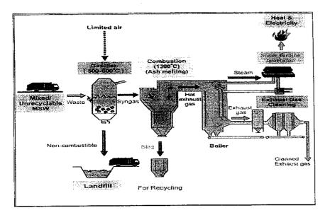
Fig.3 Process flow diagram of Close-coupled Gasification-combustion
