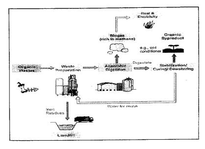
Fig.7 Process flow diagram of Anaerobic Digestion
