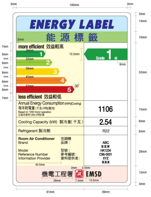
2. The dimensions of the energy label must be as specified in the diagram below –
