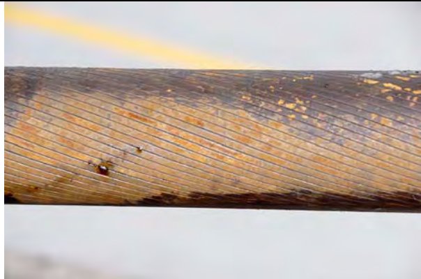
Fig. 6: Rust at the carrying rope within the range of Nei Lak Shan Angle Station
