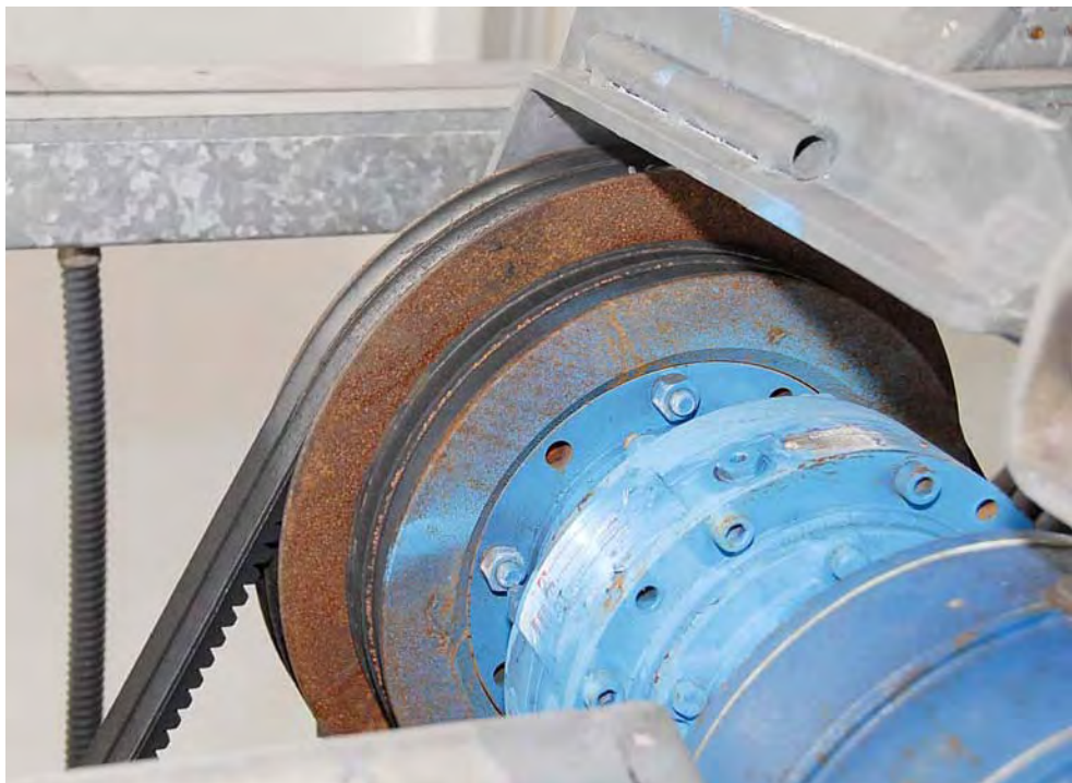
Figure 17 – Close up view on the rusty v-belt pulley
