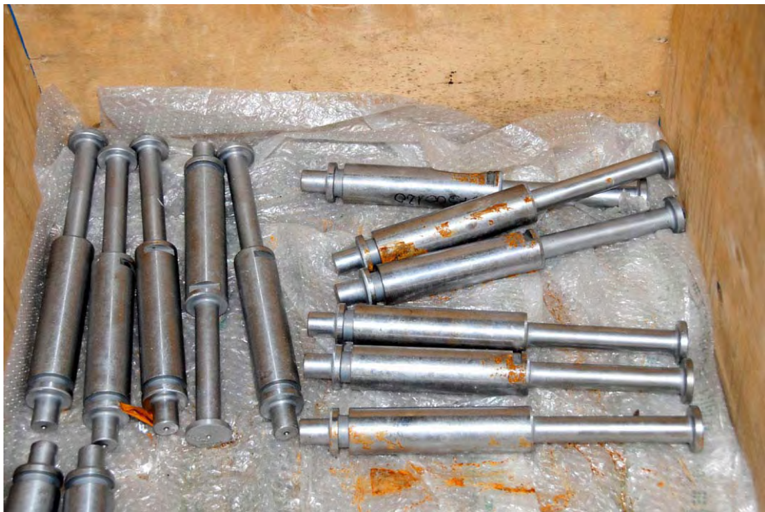
Figure 19 – Spare parts stored inside cabin storage area with sign of rust
