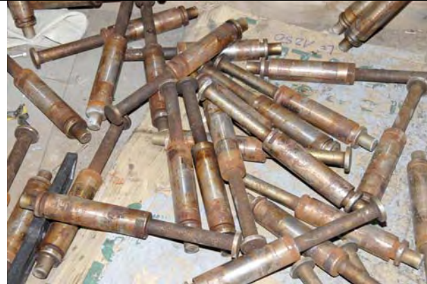
Fig. 10: Rusty axles of the connection of suspension and cabin
