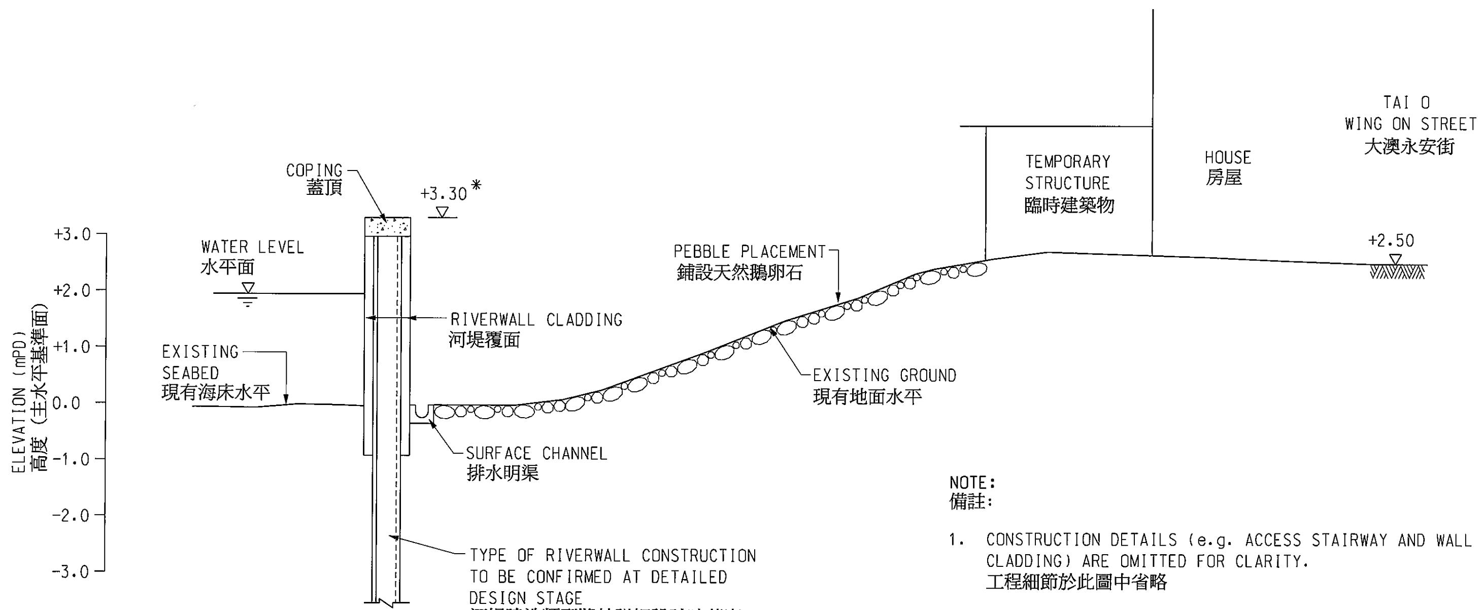
\* COPING LEVEL TO BE CONFIRMED AT DETAILED DESIGN STAGE
