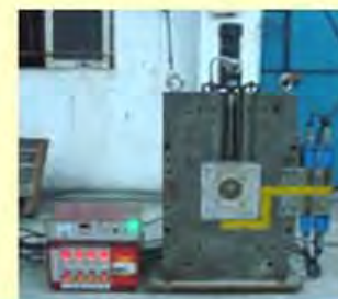
The Co-injection manifold
