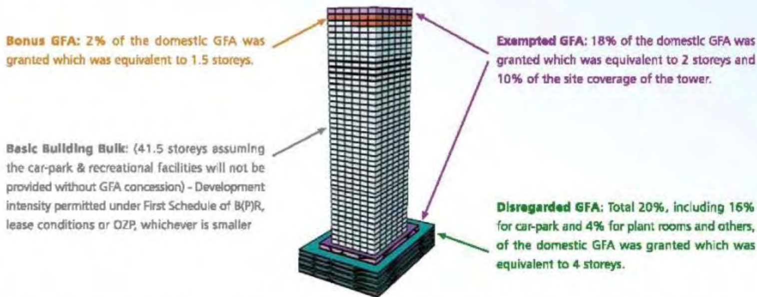
Figure 4 – Three types of GFA concessions and how they affect building bulk and height
