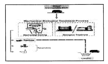
Fig.5 Process flow diagram of MBT
