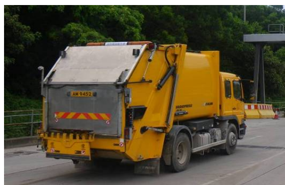
Figure 2 - Enclosed type of refuse collection vehicle (with tailgate cover) used by FEHD
