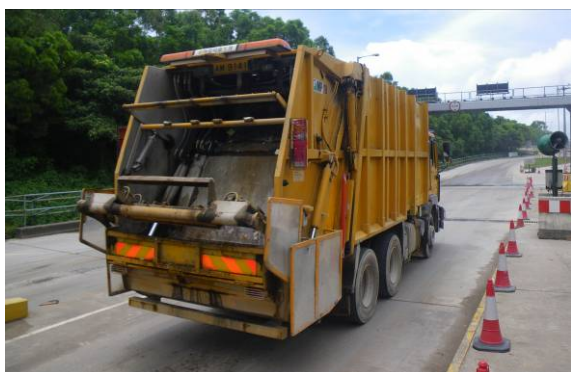
Figure 3 - Enclosed type of refuse collection vehicle (without tailgate cover) used by FEHD
